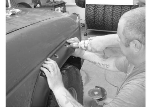
4. After cutting the wing offer up the arch and hold in place, using a 2mm drill bit drill through the middle of the arch screw recess's. This is a 2 person job to ensure accuracy.
